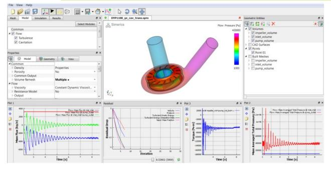
Figure 4. CFD model of Dredge 1100 (surface pressures and x-y data plots)
