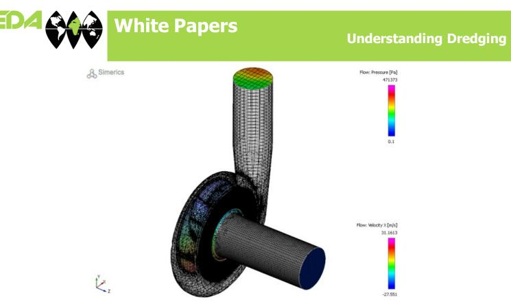
Figure 6. An illustration of the output of the pressure and velocity field from SimericsMP
