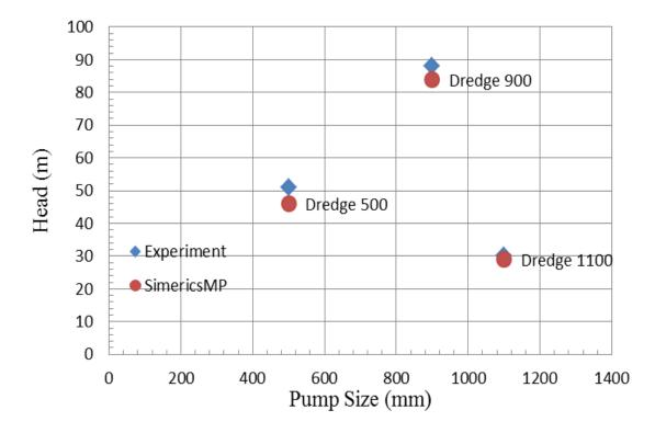
**Figure 5.** Comparison of the head predicted by SimericsMP transient simulations and the tests for three Dredge Yard pumps of different sizes: Dredge 500, Dredge900, and Dredge 1100, under the same operating conditions respectively for each pump.
